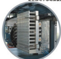
Preform mold and outside cooling Robot 瓶胚模具及模外冷却手爪
