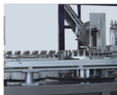
Servo cylinder preform sending and separating system 伺服瓶胚传送及分开系统
