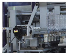
Servo bottle turning system 伺服瓶子翻转系统
