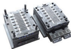
12 Cavity Hot Runner Spoon Mold 一出12热流道勺子模具
