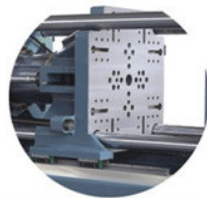
No contact between 4 tie bars and moving template linear guideway 哥林柱与中移动模板脱开不蹭蹭直线导轨
