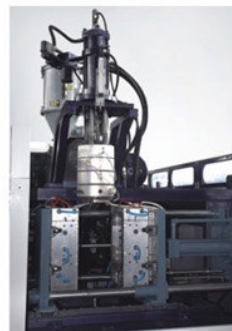
Accumulator die head 储料式模头
