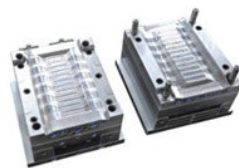
12 Cavity Hot Runner Fork Mold 一出12热流道叉子模具
